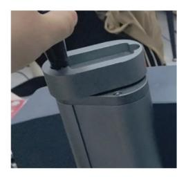
3. Use the provided ruler to measure the distance from the bottom line of the scanning head to the surface of the test material. Make a note of the distance for future reference.
