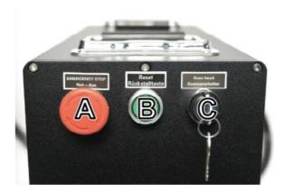
A. Emergency Stop—Because of the risk of fire and other hazards during engraving, this engraver includes a large and easy-to-reach emergency stop button near the control panel. Release it first during startup. Press it down to stop the laser instantly.
