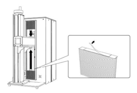
**Step 11.** Attach the interlocks to the part of the cover as shown. Peel off the backing of one interlock and press the adhesive side firmly against the indented part of the cover from inside, being sure the trigger of the interlock protrudes completely from the cover. Repeat the process for the other interlock.
