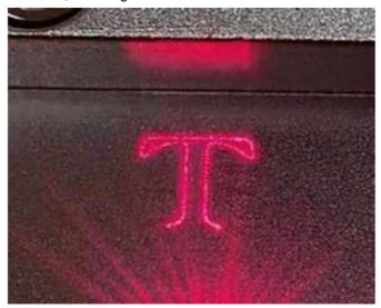
Step 7. Place an expendable piece of the material to be engraved in the location shown by the laser guidance. Do
