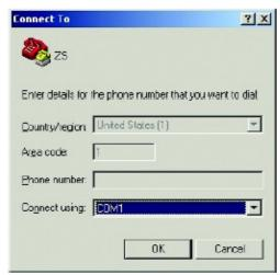
2. Select the COM port connected to the ZS in the Connection Method section.
