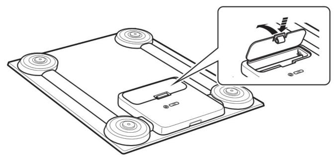
2. Install the batteries following the correct polarities as shown to the right and inside the battery compartment.
