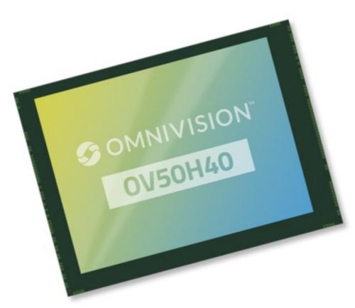
OV50H is a high-resolution 50 megapixel (MP) image sensor with a dual conversion gain (DCG) technology powered 1.2-micron (pm) pixel in a 1/1.3-inch optical format, designed for high-end smartphone rear-facing cameras. The OV5OH offers flagship-level low-light and autofocus performance, supports 12.5MP at 120 frames per second (fps) and high dynamic range (HDR) at 60 fps and is OMNIVISION's first sensor to feature horizontal/vertical (11/V) quad phase detection (QPD).
