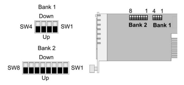
The functions of DIP-switch Bank 1 are shown below.
