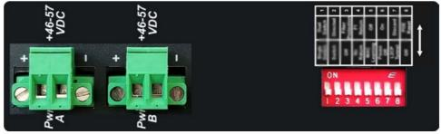
**WARNING:** OnlyaDC power source that complies with safety extra low voltage (SELV) requirements can be connected to the DC-input power supply.
