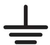
The Power Station must be grounded. Never operate it without a properly installed ground conductor.
