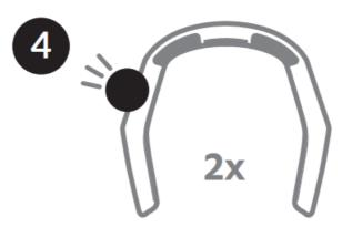
Double tap the device to wake it up (confirmed by a double vibration) – at this point the device is ready to use.
