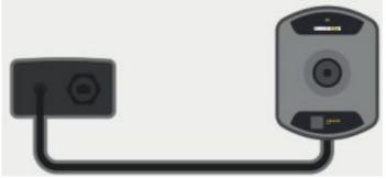
2. For IP65, use the provided IP65 connector sleeve for the RJ45 connector.
