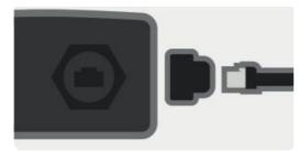
Remove RJ45 connector, apply provided IP65 sleeve. Shrink a new RJ45 connector to the Ethernet cable.
