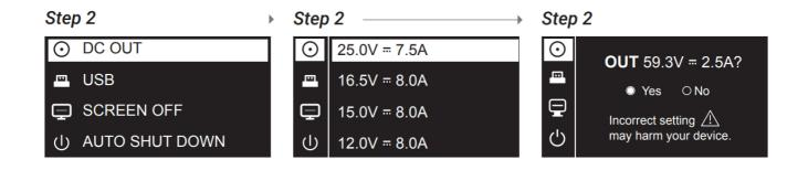
Omnicharge keeps 4 voltage presets. You can press and hold the power button while selecting a preset to customize the voltage and amperage.
