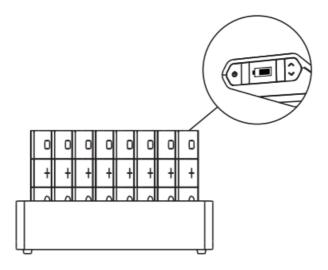
**Note**: The chargers require no force when connecting them to the charging bay. Make sure the charger is level when pushed into the slot and not crooked. Never force the Portable Charger into the charging base.
