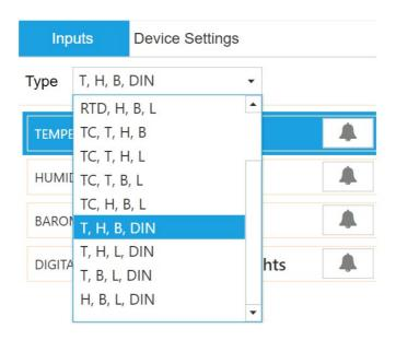
The SS-002-0 offers a configurable choice of one external thermocouple, RTD, or DIN (contact closure). The SS-002-1 offers a configurable mix of any three of the four internal sensors: Temperature, Humidity, Barometric Pressure, Ambient Light, AND one external sensor option: Thermocouple, RTD, or DIN (contact closure).
