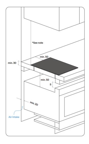
IMPORTANT: Regarding adjacent walls, cupboards and protection for combustible materials: Always ensure that the appliance is installed in accordance with AS/NZS 5601.1, or AS/ NZS 5601.2 with regard to clearances to combustible surfaces and materials, and clearances to rangehoods and exhaust fans.
