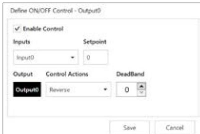
Figure 10: Configuring On/OFF Control
