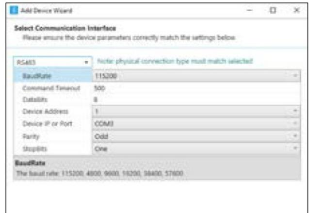
Figure 4: USB and RS485 Communication Interface
