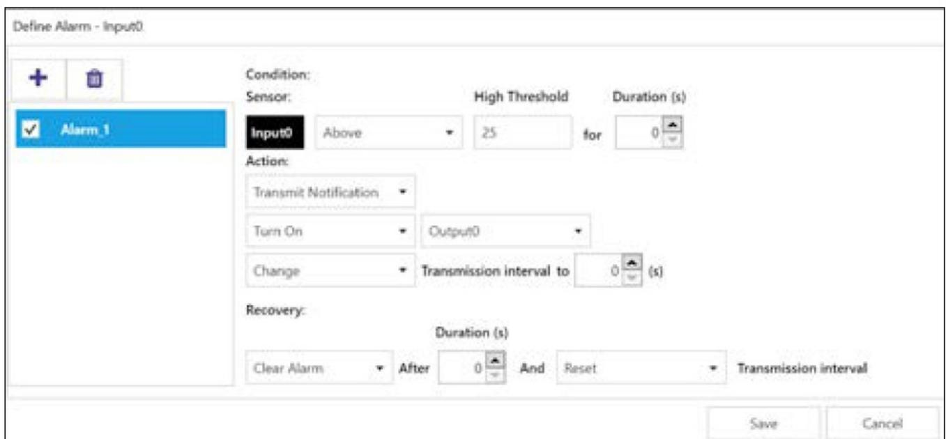
The screenshot shows the 'Define Alarm - Input0' dialog box. On the left, there is a list of alarms with 'Alarm\_1' checked. The main configuration area is divided into sections: 'Condition' (Sensor: Input0, Above, High Threshold: 25, Duration (s): 0), 'Action' (Transmit Notification, Turn On: Output0, Change: Transmission interval to 0 (s)), and 'Recovery' (Clear Alarm, After: 0, And: Reset, Transmission interval). 'Save' and 'Cancel' buttons are at the bottom right.
