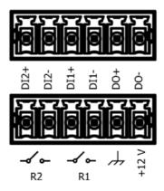
**Important:** When wiring the included terminal block connector to access the digital I/O, alarms, or relays, it is recommended that users ground the unit by connecting a wire to the chassis ground of the connectors shown in the diagram above.
