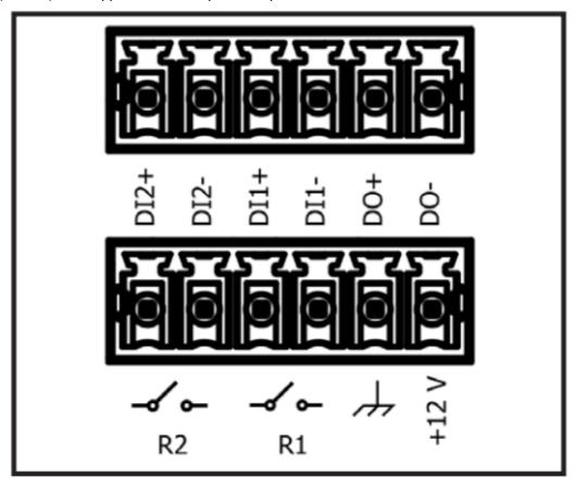
Important: When wiring the included terminal block connector to access the digital I/O, alarms, or relays, it is recommended that users ground the unit by connecting a wire to the chassis ground of the connectors shown in the diagram above.
