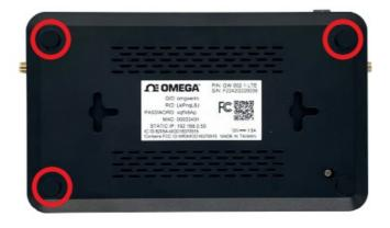
**Step 2:** Unscrew all four screws indicated in the figure below. The user may then remove the top cover of the GW-002 device casing.
