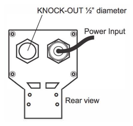
On sensor-mounted units, the output signal wires must be installed through the back panel using a second liquidtite connector (included). To install the connector, remove the circular knock-out. Trim the edge if required. Install the extra liquid-tite connector.
