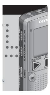
• When the NOISE CANCEL switch is set to ON, playback speed returns to normal.
