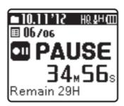
To pause recording, press the REC (O) button while recording. To resume the recording, press the REC (O) button again.
