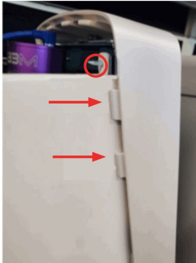
Figure 20. Aligning pin and bezel tabs
