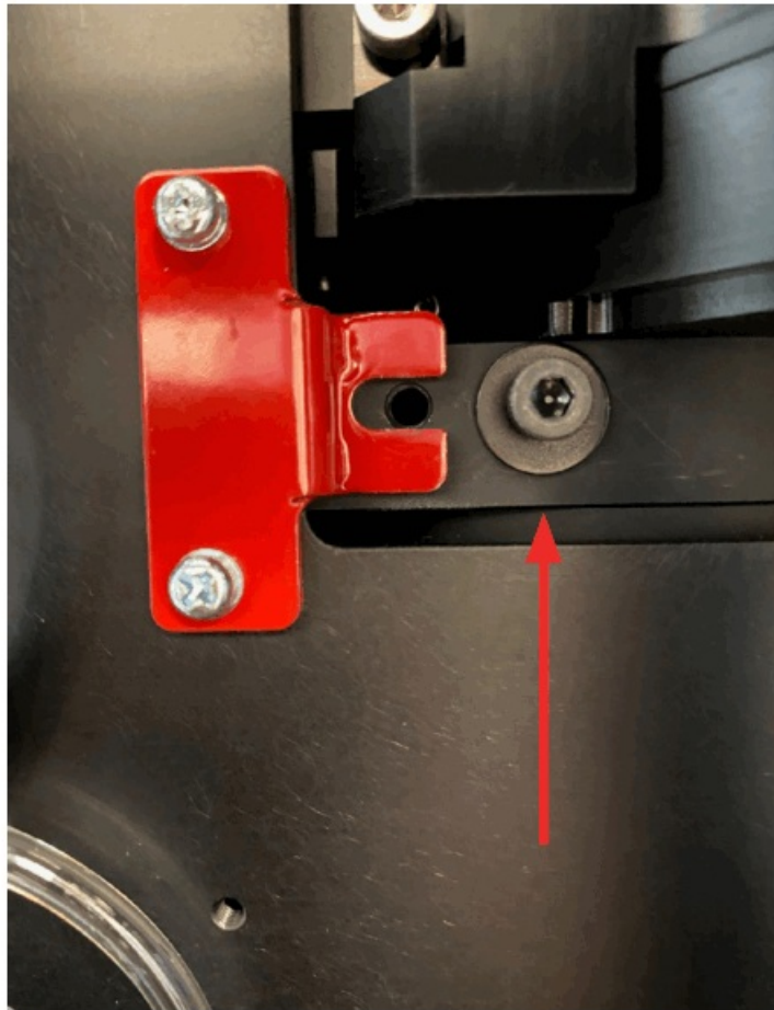
Figure 17. Shipping lock screw moved to "run state", i.e. not to be used during shipment
