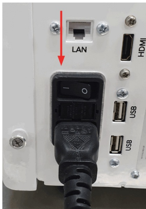
Figure 24. Instrument power switch toggled on
