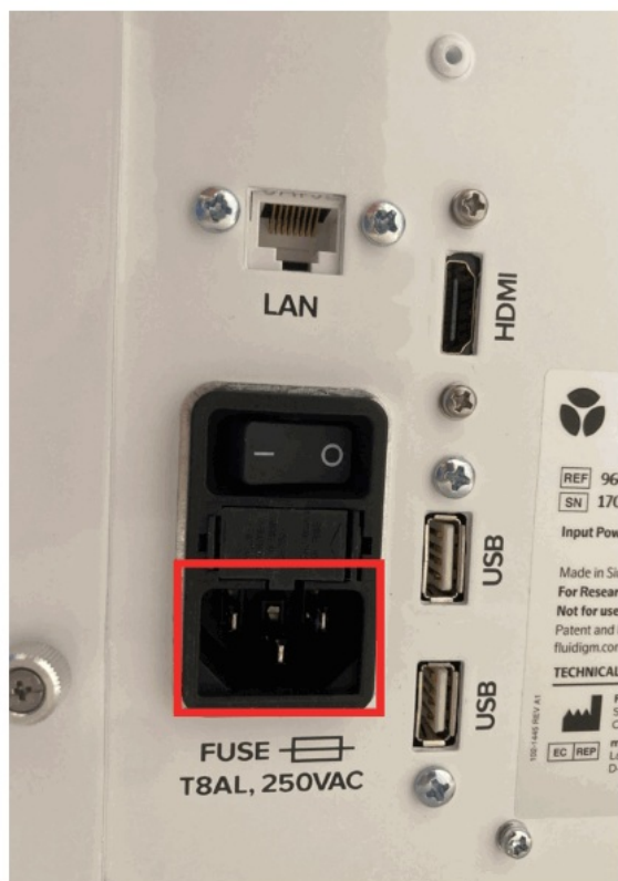
Figure 23. Power cord connection
