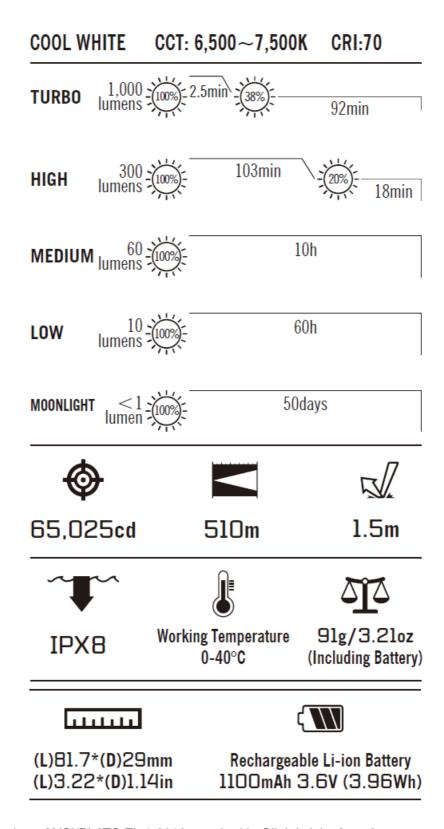
Above data are tested per ANSI/PLATO FL 1-2019 standard in Olight's labs for reference.
