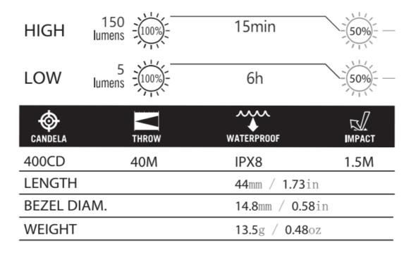
**NOTE:** The output brightness will decrease as the battery power decreases. The running time is the time when the brightness attenuates to 50% of the
