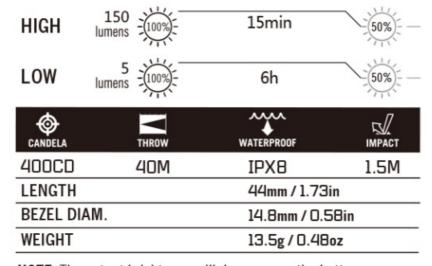
**NOTE:** The output brightness will decrease as the battery power decreases. The running time is the time when the brightness attenuates to 50% of the initial value after the battery is fully charged.
