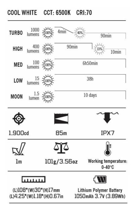
The above data are tested per ANSI/PLATO FL 1-2019 standard in Olight's labs for reference.
