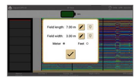
Finish the scan after scanning the last line, enter the scan field dimensions and save it for further analysis.
