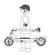
③ Hold the steering tube to lift the electric
