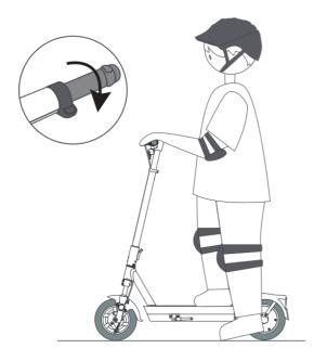
4. Release the acceleration handle to reduce speed, and squeeze the brake lever to brake.
