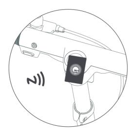
**NFC card**: when powered off, put the NFC card close to the screen to turn on and unlock the scooter; When powered on, place the NFC card close to the screen to shut down and lock the scooter.
