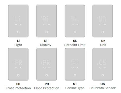
**LIGHT**In the Light setting, you can set the brightness level for the screensaver and the active screen.
