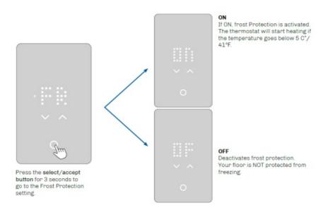
You have the option of setting the thermostat in standby mode so that only frost protection is activated if enabled. All other functions in the thermostat are switched off. Frost protection means that the thermostat activates the heating when the sensor measures a temperature below the frost protection limit.
