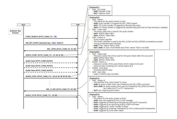
Note: The "On-request" assistant interaction model must be supported by all Remote Control and it should be used by default before any other interaction model is negotiated by GET\_CAPS, CAPS\_RESP messages exchange.
