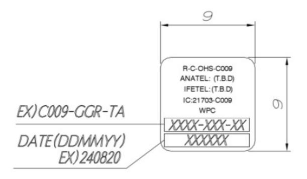
It is attached to the PCB and it can be seen into the battery compartment after removing the battery cover.
