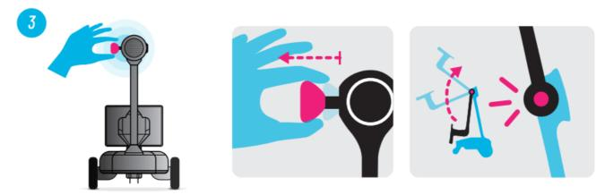
4. Pull/roll Ohmni up against the dock making sure the silver charging pins on Ohmni make contact with the charging contacts on the dock (listen for the click). The charging dock will turn blue indicating charging.
