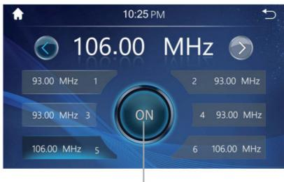
ON Click "ON" to turn on the radio transmitter, set a random frequency band, then use the car radio searches for the corresponding band to synchronize audio.
