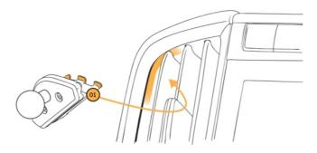
3. Using the L-key, hand tighten the screws until the mounting base has a snug fit. To ensure the best fit possible, hold mounting base while tightening.
