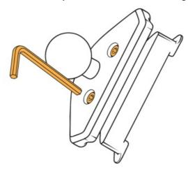
2. Position mounting base into the upper outer corner of the center console air vent. Ensure the tabs on the rear mounting base plate engage the lip behind the air vent bezel (01).
