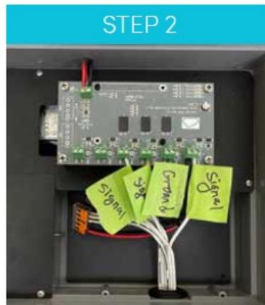
**Disconnect PCB Wires**
