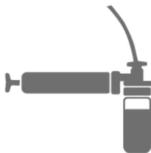
Remove the tube after draining and wipe it. Disposal of the tube and cloth. Unscrew the sample bottle and place it on a horizontal surface.
