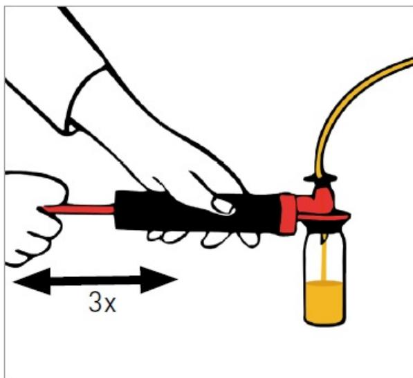
If the screw connection is tightened and the sample bottle is screwed on, but no vacuum is created, the small valve ball is likely to be missing. This could happen when the pump was opened during cleaning on a previous occasion.
