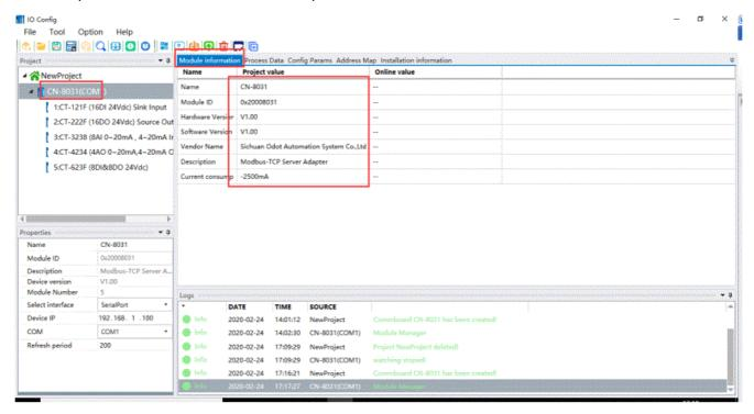
**In the Process Data interface**, you can view the data type of the IO module, as well as the online monitoring value of the input data, and the online monitoring value and the current value of the output data.
