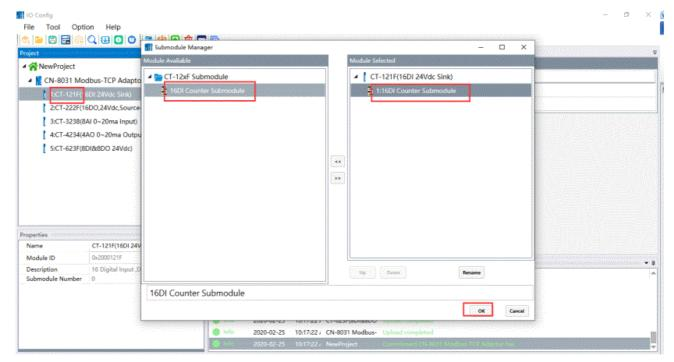
After adding a sub-module, you must right-click to download the module configuration or right-click CN-8031 to download IO parameters. Otherwise, if clicking directly online and it will result in an error in the state menu of "the number of sub-modules does not match the total number of configuration sub-modules".
