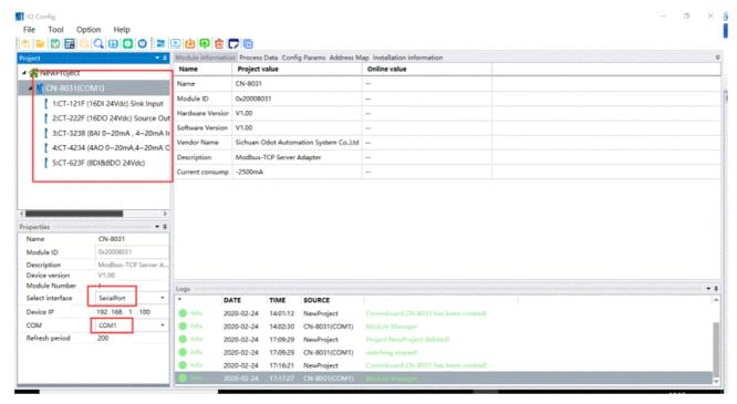
Module manually adding supports shortcut keys "Ctrl C", "Ctrl V" and "Delete" for copy, paste and delete IO module. Select CN-8031 and click the shortcut "Ctrl S" to save the configuration project.
