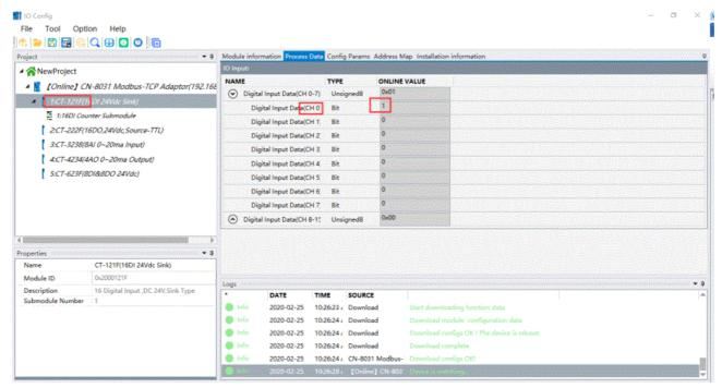
**Example**: Assigning the CH0 channel of CT-4234 in slot 4 to 16#7530= 30000, and connect it to the CH0 channel of CT-3238 in slot 3 at the same time. The CH0 of CT-3238 monitoring value is 16#3125.
