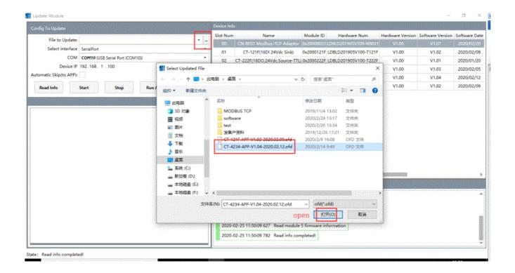
The upgrade version and other information could be viewed in the lower left side of the upgrade menu. And there is no upgrade for the currently firmware version so no need for upgrading. If the version information is inconsistent, please select the slot where the module is located(marking  $\sqrt{}$ ) and click to start the upgrade.
