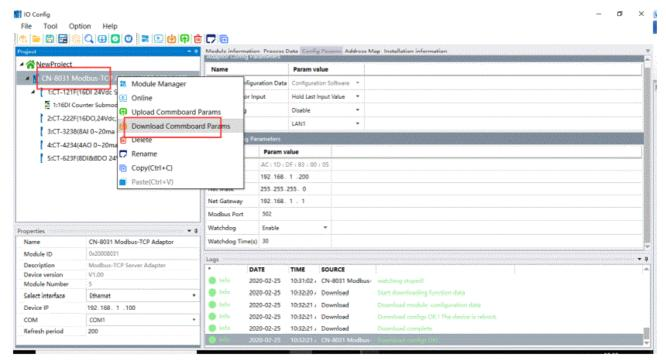
After all parameters are modified, select CN-8031 and click the shortcut key "Ctrl S" to save the configuration project.
