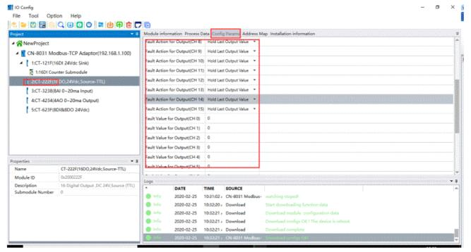
After the parameters are changed, you can right-click on CN-8031-Download IO Parameters in the project bar. So the configuration parameters of the adapter and IO module could be modified.
