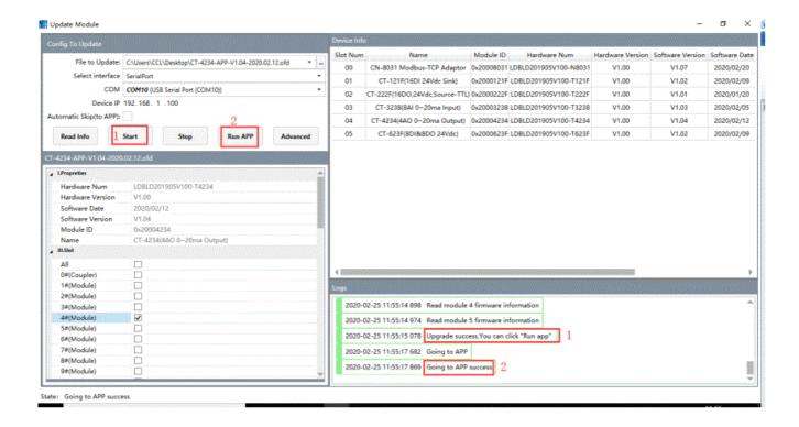
If it only needs to upgrade the firmware of one module, you can select Automatic Skip (to APP), and click Start for upgrade, then the APP will run automatically when the upgrade is completed. If it needs to upgrade the firmware of multiple modules, please do not select Automatic Skip (to APP). Clicking Run APP after all the modules upgrade is finished.
