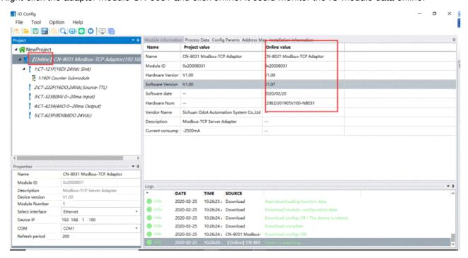
**Example**: CT-121F in slot 1, the external power 24VDC is supplied to the DI0 of CT-121F. And in the process data interface, the CH0 monitoring value is 1.
