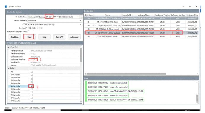
Please note when upgrading: just click to Start for the upgrade, after the upgrade is completed, and it requires to enter APP mode, so it needs to manually click "run APP" or power up the device again.
