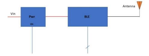
The transceiver Tx power is: -20 to +4 dBm The section is powered typically at 4.2V
