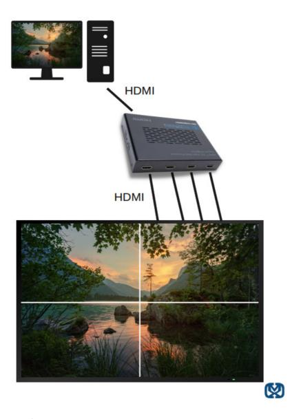
8 Video Wall Configurations: Splitter configurations built into the 4K video wall processor:  $2 \times 2 \mid 1 \times 2 \mid 2 \times 1 \mid 1 \times 3 \mid 3 \times 1 \mid 1 \times 4 \mid 4 \times 1 \mid$ . The flexible wall configurations allow users to transform their space without compromise.
