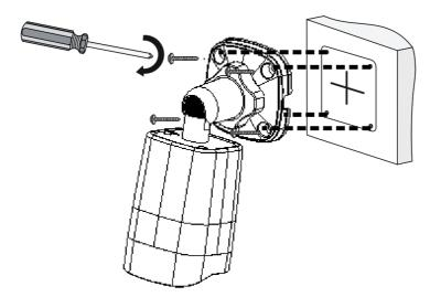
Lead tapping screws through the guide holes in the base and fix them on the wall by using a screwdriver.
