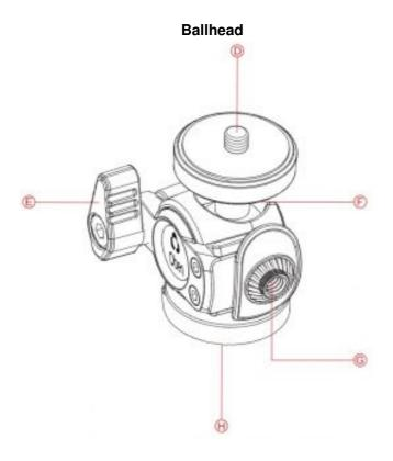
**D:** 1/4-20 screwAttach to smartphone adapter.
