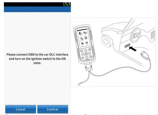
③ Click [Confirm], the device automatically read the sensor ID saved in the device board and display it on the screen.
