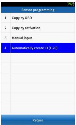
2 Place 1-5 QQr sensors within 10cm of the tool; The instrument automatically detects nearby sensors.
