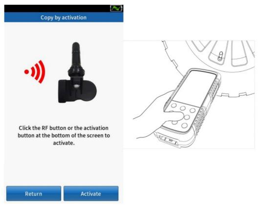
③ If the activation is successful, the OE sensor ID is displayed at the bottom of the screen.
