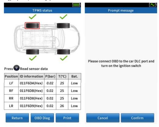
② Connect the OBD cable to the vehicle DLC interface, and turn on the ignition switch.
