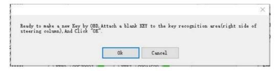
③Put the New Key Close to the Vehicle Induction Coil to Ensure That the Current Key ID Is Not in the Vehicle Key List.
