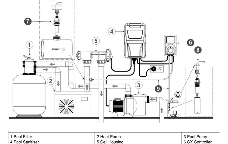
7 Injection with Tee 8 Suction with Drum weight & label 9 PVC Flexible Tube
