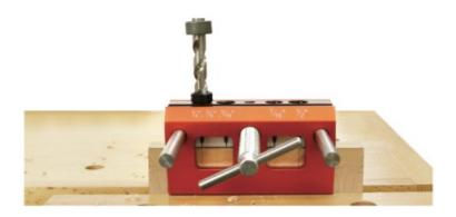
Put the drill bushing into the guide hole of the correct size, and insert the drill bit that meets the size to drill the required depth. Repeat the same process on the other board.
