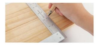
Mark the center marking line for the dowel holes to be drilled on the two boards to be connected.
