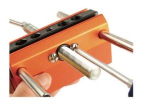
**Step 3.**Pull the locking plate towards the centerpiece for clearance to adjust the adjuster nut.
