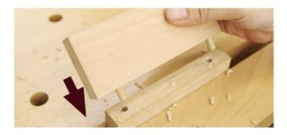
Apply glue to dowels and hole. Insert the dowels in one board, then put in another board , and clamp securely until dry.
