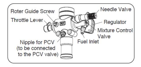
Two adjustable controls are provided on this carburetor.
