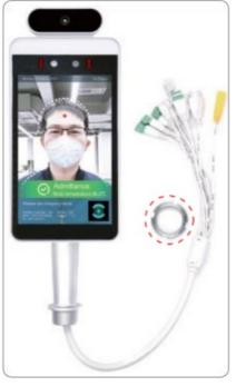
③ Under the gate, insert the cable and cable interface into the gasket and nut, in turn, tighten the nut, connect the power supply, and the screen will start.
