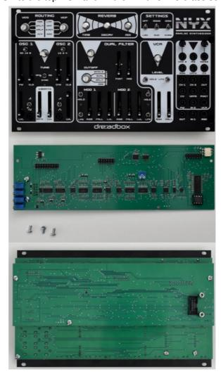
6. Step 6 Attach the power board to the assembly as shown and secure with 2xM3 brass screws.
