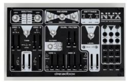
11. Step 11 Screw the knobs to the pots and rotary switches as shown.
