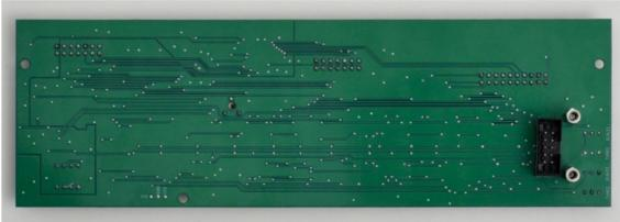
5. **Step 5** Connect the bottom PCB to the top PCB and fix them with 3xM3 brass screws as shown.
