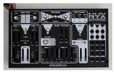
10. **Step 10** Screw in the pots and rotary switches, taking care that the rotary switches should not be overtightened but not too loose. The M10 nuts are for the rotary switches and the M8 for the pots.
