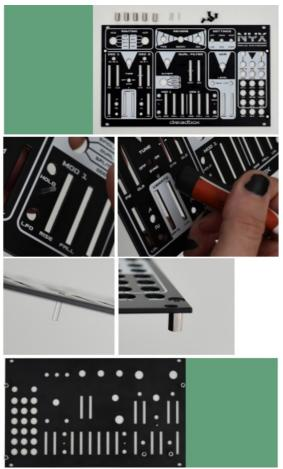
2. Step 2 On the top PCB above the 2nd slider to the right as shown in the picture, add an M3 brass screw
