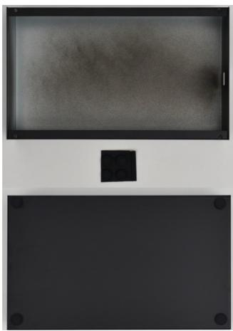
8. **Step 8** Place the unit in the metal enclosure. To easily achieve this, place the unit with the USB side first, and then push down the rest.
