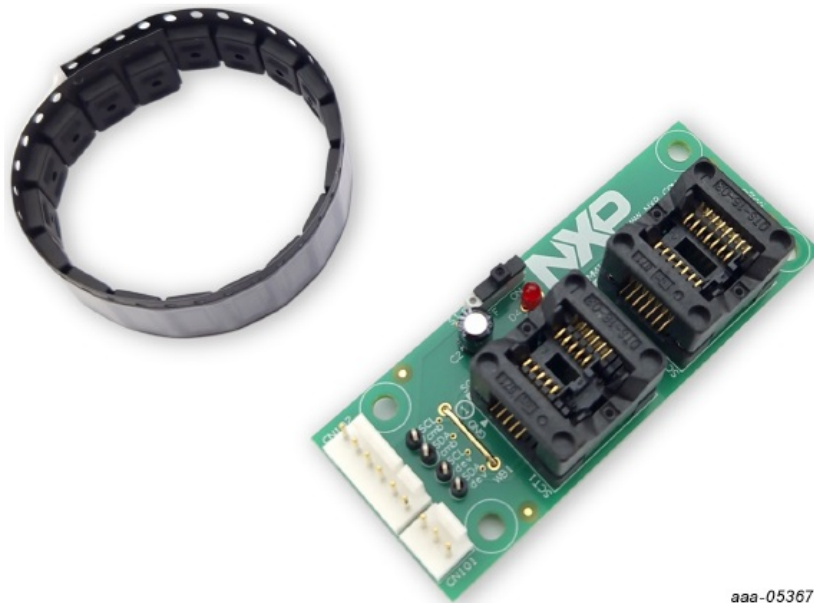
Figure 2. 20 TEA2376DT samples and a TEA2376DB1604v3 programming board
