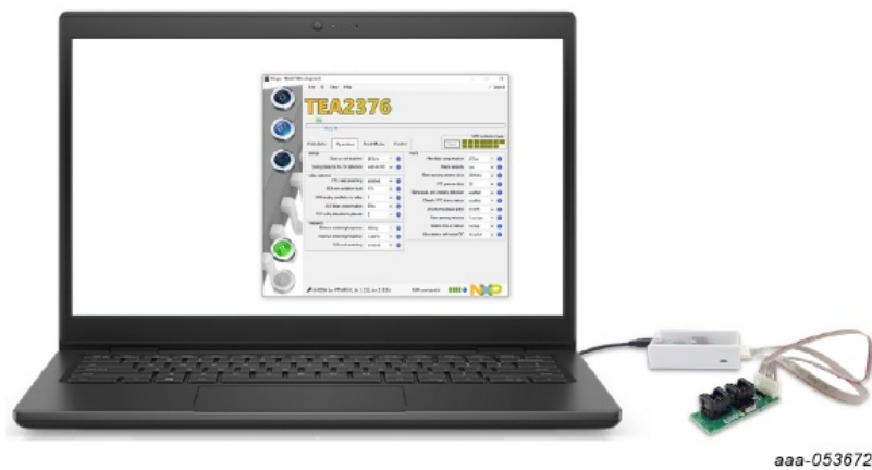
Figure 4. Setup for programming with the Ringo software on a PC
