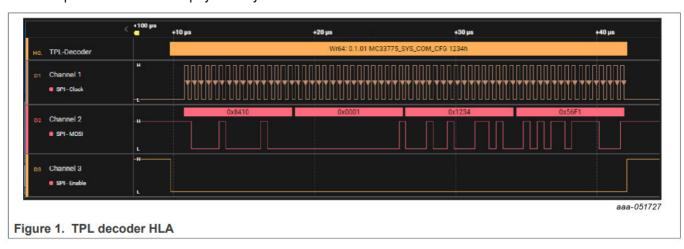
This tool is also part of the NXP battery management system (BMS) communication decoder ecosystem and can work together with the KIT-TPLSNIFEVB hardware board that facilitates the acquisition of electrical transport protocol link (ETPL) signals.
