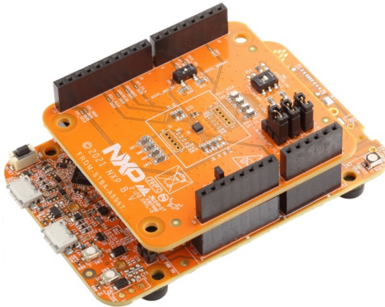
Figure 1. FRDM-STBA-A8967 attached to FRDM-K22F MCU board
