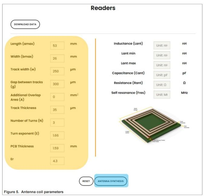
Step 4 – Check the calculated parameters.
